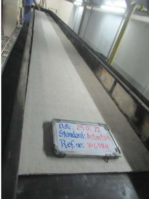
Photo 1: Specimen before the test. (Non-Fire Side)
