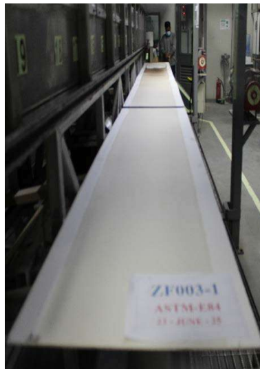
Photo 4: Specimen after the test. (As seen from the exhaust end)
