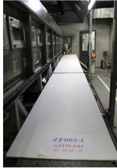
Photo 2: Specimen before the test. (Fire Side)
