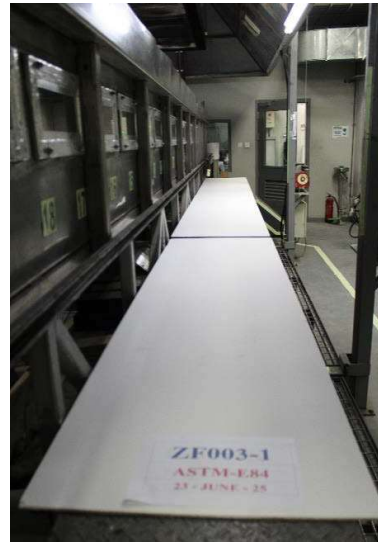
Photo 2: Specimen before the test. (Fire Side)
