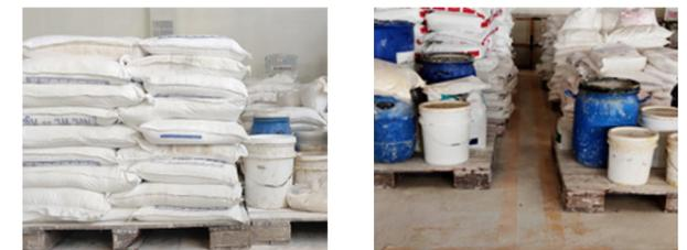
Before Single line marking to separate batches      After Double line marking to separate batches
