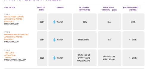
APPLY ULTIMA PROTEK BASE COAT (SELF PRIMING + 1 UNDILUTED COAT) + THREE COATS OF APEX ULTIMA TOP COAT AS PER THE RECOMMENDED APPLICATION PROCEDURE ON HORIZONTAL SURFACES LIKE TOP OF WINDOWS/CHA11AS ETC
